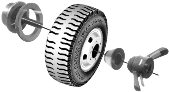
Put together the large flange to the matcher - wheel - large cone - quick nut
